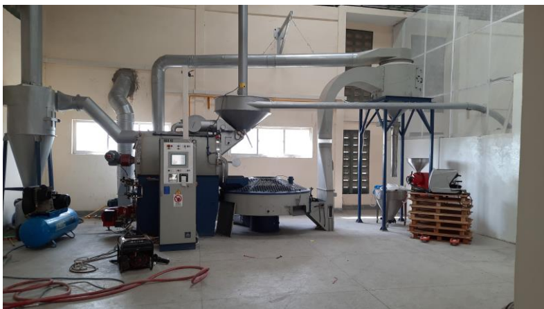
Figure 3 Modern Roaster with 120KG/Batch capacity
